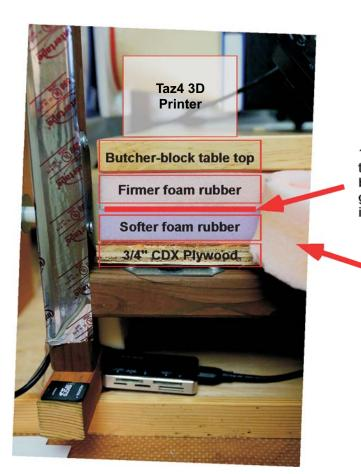
18Ga sheet metal, between the foam sheets, trimmed so the sharp edges are not accessible. Consider taping any sharp edges. I used galvanized steel, but aluminum is fine; it's the in-plane shear resistance we're after.
